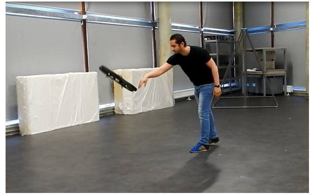
Fig. 3. One of the members of our team pushing the UAV to generate a disturbance in flight experiments.
