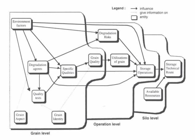
Fig. 1. The relations between the entities present in the space of the storage technical route
