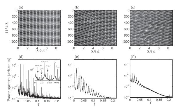
FIG. 3. Space-time diagrams and frequency power spectra of pattern states for E = 0.011: (a, d) ribbons without defects for Ta = 49.05; (b, e) ribbons with defects for Ta = 50.1; (c, f) spatio-temporal intermittency regime for Ta = 54.82. The inset of Fig. 3(d) represents a zoom of power spectrum in the neighborhood of fundamental frequency.
