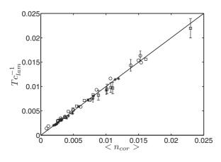
FIG. 10. Variation of the characteristic laminar time with the corrected mean defect number for the three values of E: E = 0.011 (stars), E = 0.020 (squares), and E = 0.046 (circles)
