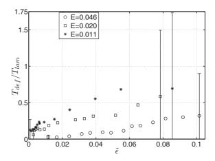
FIG. 11. Variation with  $\tilde{\epsilon}$  of the ratio of the mean lifetime of defects to the mean laminar time of defects for the three values of the elasticity number, E = 0.011 (stars), E = 0.020 (squares), and E = 0.046 (circles). The error bars represent the standard deviations
