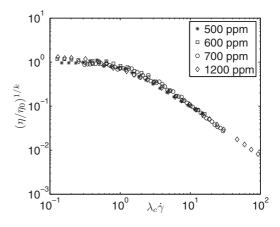
FIG. 1. Master curve of the variation of the dynamic viscosity of polymer solutions of PEO in 95% water–5% isopropyl alcohol with the dimensionless shear rate  $\lambda_C \dot{\gamma}$  for three working concentrations.
