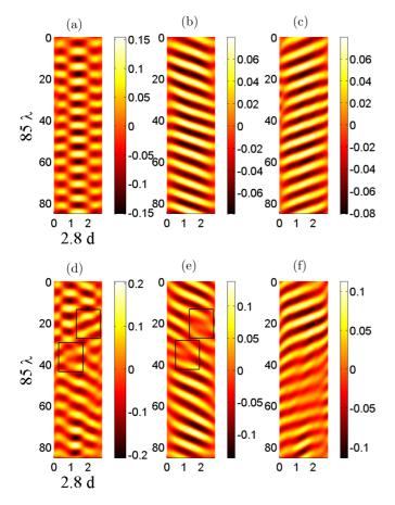
FIG. 5. Spatiotemporal diagrams of the radial velocity component for ribbon state without defects (a) for Ta = 41.9 and with defects (d) for Ta = 46. Spatiotemporal diagrams of the the right (b, e) and left (c, f) spirals for ribbons without defects and with defects. The velocities are scaled by  $d/\lambda$ . The data correspond to a working solution with E = 0.137.
