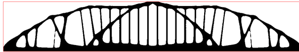
Figure 4: Optimized design \Omega^* for the variant (11) of the constrained shape optimization problem (10).
