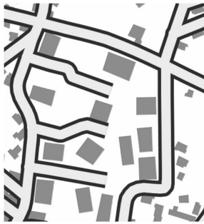
Figure 2. Example of dead-end road gliding with its neighborhood in order to liberate room between it and the southernmost other dead-end. Top left: initial situation. Bottom left: the buildings were enlarged and partially suppressed, and dead-ends glided. Top right: the interaction matrix for the urban block environment. Bottom right: schemas of relations between agent type (plain arrows mean 'situated in').
