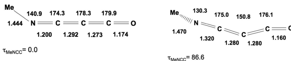
FIG. 2. Calculated “linear” and “bent” structures of Me-NCCCO ( 1a and 1a' ) at the LCCSD(T)/cc-pVTZ level (bond lengths in Å; bond angles and dihedral angles \tau in degrees (°)). The energy difference between 1a and 1a' is \Delta E = 0.03 \text{ kcal mol}^{-1} . The energy barrier for linearization in 1a' is 3.1 \text{ kcal mol}^{-1} .
