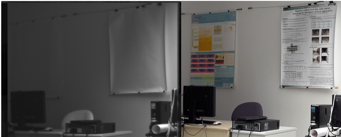
Figure 3. Serigraphy in visible and infrared spectra: whereas the printed shapes are discernible in the visible spectrum, the posters seem blank in the infrared spectrum.
