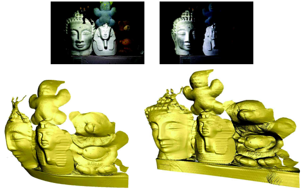
Figure 4. Top: two out of m = 8 RGB images recorded under nearby lightings. Bottom-left: reconstructed shape using the directional lightings and the orthographic projection models. Bottom-right: rendering of the shape reconstructed using the pointwise lightings (18) and the perspective projection (13) models, seen under the same angle.
