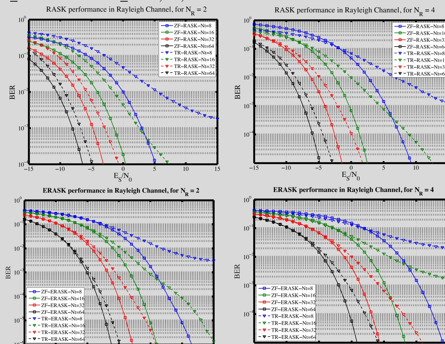
For low complexity receivers, ZF preprocessing outperforms MRT Interference cancellation detectors could be used for better performance with higher cost of complexity
