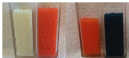
Figure 2. On the left, Marathon ® resin in HNO 3 1M, on the center, Marathon ® resin with only 10% of its sites occupied by TazoC, on the right the same after contact with a concentrated solution of Pd(II).
