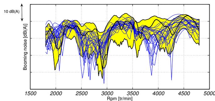
**Figure 3.** The horizontal axis is the engine rotation expressed in rotations per minute corresponding to the frequency band [50,160] Hz. The vertical axis is the level of the acoustic pressure in dB(A). Experimental measurements (20 blue thin lines). Prediction with the ROM (black thick line). Prediction with the identified SROM of the confidence region corresponding to the probability level 0.95 (region in yellow color of in gray). Figure from [110].
