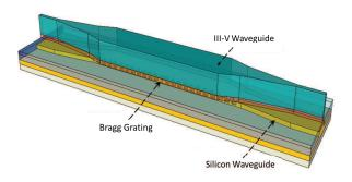
Fig. 1. Hybrid III-V/SOI DFB laser structure.
