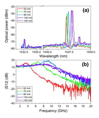
Fig. 5. (a) Optical spectra of the hybrid DFB laser for different bias currents and (b) the corresponding small-signal amplitude modulation responses.
