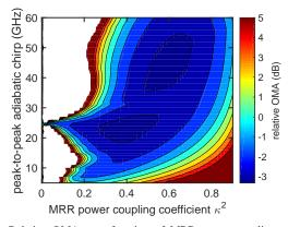
Fig. 3. Relative OMA as a function of MRR power coupling coefficient  $\kappa^2$  and peak-to-peak adiabatic chirp of the DML: negative values show the improvement provided by the MRR. The calculations have been performed here with  $\alpha=2$ , but since the peak-to-peak adiabatic chirp depends on the product  $\alpha\kappa_c$ , the actual value of the linewidth enhancement factor does not significantly impact the results.
