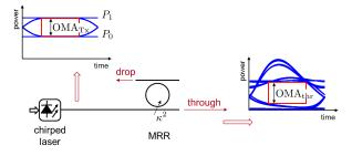
Fig. 2. MRR optimization procedure based on comparison of the OMA at the DML output (OMA<sub>Tx</sub>) to the OMA after filtering at the through port of the MRR (OMA<sub>thr</sub>) for different values of peak-to-peak adiabatic chirp and MRR power coupling coefficient  $\kappa^2$ .
