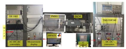
Figure 9 : Hardware-in-the-loop experiment benchmark
