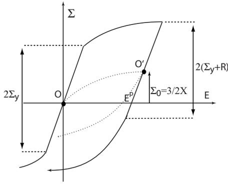
Fig. 3. Kinematic and isotropic variables identification in a classical stress-strain diagram.
