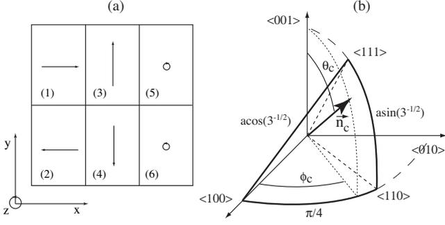
Fig. 2. (a) Initial domain structure of single crystal considered for the multidomain modeling; (b) standard triangle and loading axis  $\vec{n}_c$ .
