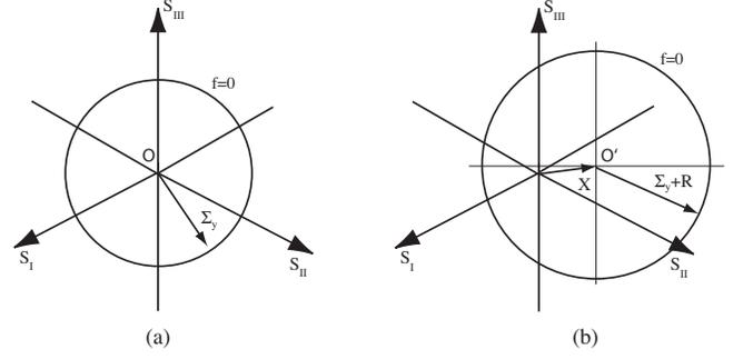
Fig. 1. Illustration of kinematic and isotropic hardening for a von Mises criterion in the deviatoric eigen-stress space ( $S_I, S_{II}, S_{III}$ ): (a) initial yield function; (b) yield function after strengthening.
