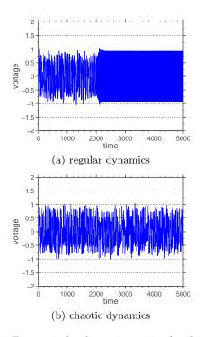
Figure 2 Two typical voltage time-series for the bistable energy harvesting system. The time-series in (a) has a regular steady-state dynamics, while in (b) a chaotic steady-state dynamics is observed.
