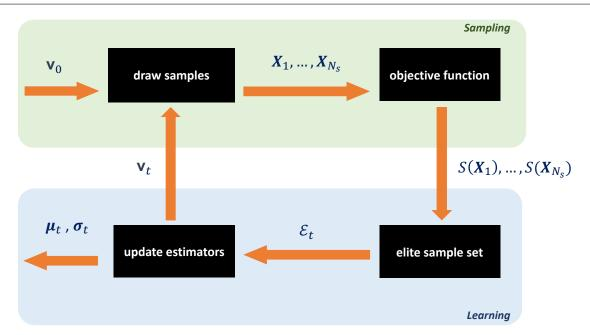
Figure 3 Schematic representation of the CE algorithm for optimization.
