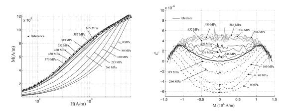
FIG. 1 – Anhysteretic magnetic (a) and parallel magnetostrictive (b) behaviors of the sample prestrained at 3% and reloaded at different stress levels
