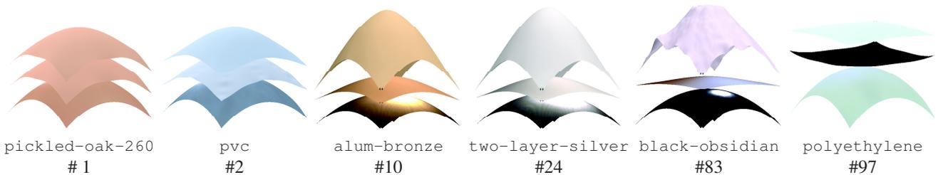
Figure 5. 3D-Reconstruction results for several materials from the MERL database, sorted according to their ranking in Figure 4. Bottom row shows the ground-truth surface and reflectance, middle row shows the shape recovered while estimating automatically  $c$  using (23). Top row shows the results with  $c = 1$ .
