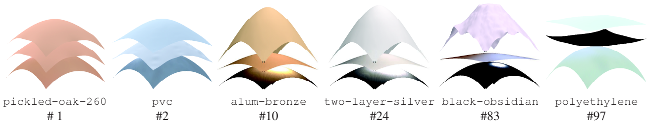
Figure 5. 3D-Reconstruction results for several materials from the MERL database, sorted according to their ranking in Figure 4. Bottom row shows the ground-truth surface and reflectance, middle row shows the shape recovered while estimating automatically c using (23). Top row shows the results with c = 1 .
