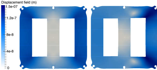
Fig. 7: Displacement field described by color density at t_1 (left) and t_2 (right). Deformed core shape is shown with a scale factor of 20000
