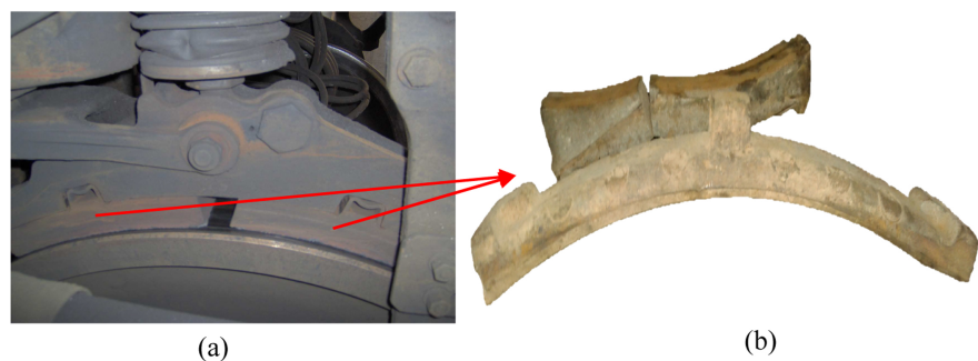
Figure 1. Braking system (a) and brake blocks (b).
