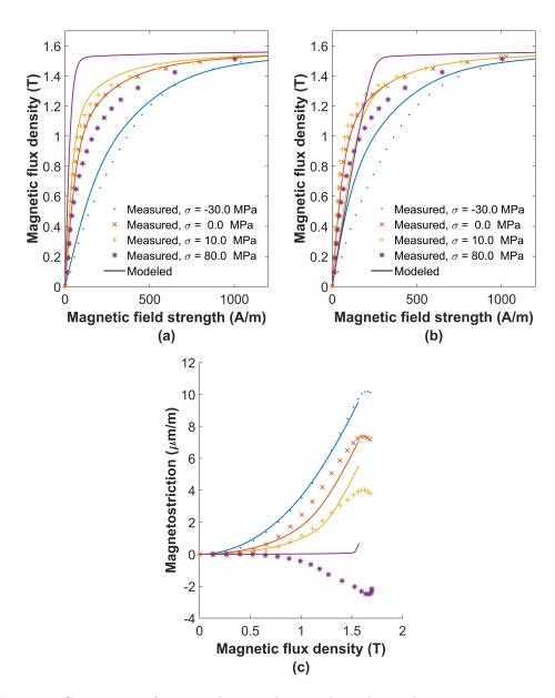
Figure 4: Comparison of measured uniaxial stress dependent anhysteretic magnetization and magnetostriction with modeled results from SM model. (a) Anhysteretic magnetization results without  $\boldsymbol{H}_{\rm conf}$  ( $\eta = 0$ ). (b) Anhysteretic magnetization with  $\boldsymbol{H}_{\rm conf}$ ( $\eta = 2.33 \cdot 10^{-4}$ ). (c) Anhysteretic magnetostriction results. (Same legend as in Fig. 4. (a) and (b))
