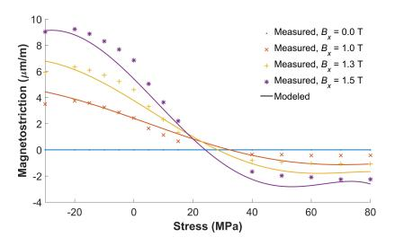
Figure 6: Comparison between modeled and measured uniaxial stress depended magnetostriction under several induction levels applied along rolling direction (x) for Material II. Modeling results are obtained from the HE model.
