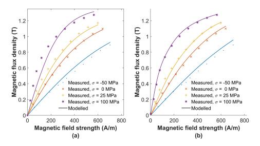
Figure 1: Comparison of measured uniaxial stress dependent anhysteretic magnetization results with modeled results from (a) SM model and (b) HE model.
