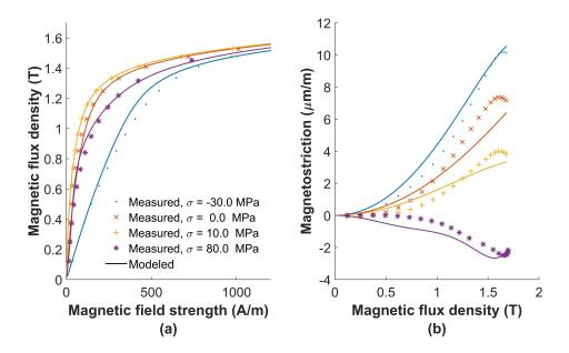
Figure 5: Comparison of measured uniaxial stress dependent anhysteretic magnetization and magnetostriction with modeled results from HE model. (a) Anhysteretic magnetization and (b) anhysteretic magnetostriction results. (Same legend as in Fig. 5. (a))
