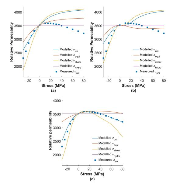
Figure 7: Permeability evolution under multiaxial magneto-mechanical loadings for Material II. Measured uniaxial permeabilities are shown with the markers. (a) SM model results without  $H_{\text{conf}}$  ( $\eta = 0$ ), (b) SM model results with  $H_{\text{conf}}$  ( $\eta = 2.33 \cdot 10^{-4}$ ), (c) HE model results.
