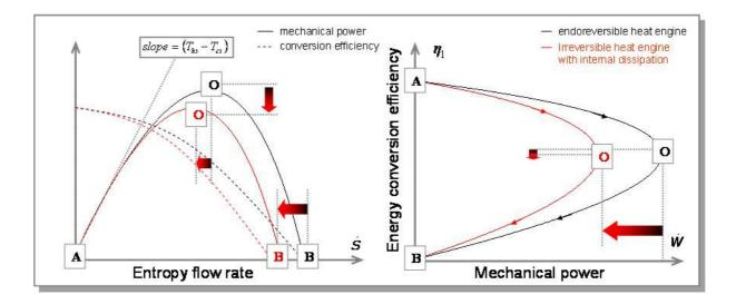
By deriving the expression (21) regarding the entropy flow rate  $\dot{s}$ , we obtain an expression similar to that obtained in the case of an endoreversible heat engine [1] where the temperatures of the heat source and the heat sink have been replaced by their apparent values [*cf.* Equation (22)]:
