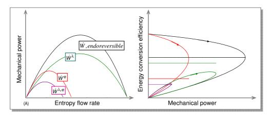
The parameter  $\zeta^{\lambda,\varphi}$  alone cannot be used to characterize the performance of a heat engine. For a given  $\zeta^{\lambda,\varphi}$ , the maximum output power may be different according to the values of  $\lambda$  and  $\varphi$  (*cf.* Figure 11). As a result, in the case of thermoelectric conversion, we should not base all the research of thermoelectric materials only on the figure of merit ZT.
