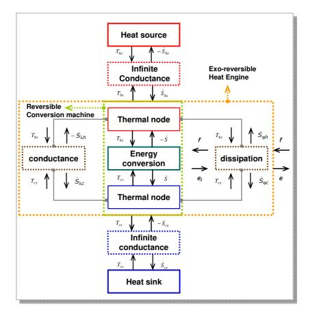
Figure 2. Bond-Graph diagram of an *exo*-reversible heat engine at steady state.
