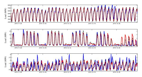
Fig. 2: CER data: measured load (blue curves) and corresponding forecast with independent (red curve) and multi-task (black dashed curve) for the aggregated demand (top panel), a single SME meter (mid panel), and a single residential meter (bottom panel). Measurements are shown over 5 weeks of the test period. All forecasts are obtained using a multiplicative kernel model (16).
