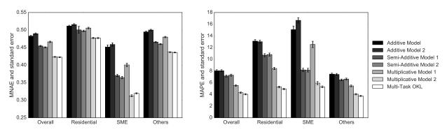
Fig. 3: Accuracy of the different medium-term forecasting methods on the CER dataset
