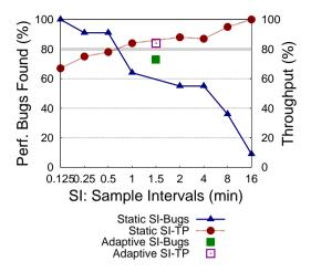
Figure 30. Critical Perf. Bugs vs. Throughput - WAIT.
