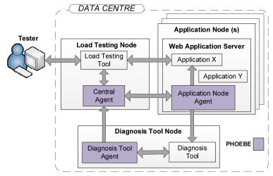
Figure 1. PHOEBE: An Automation Framework for Performance Testing
