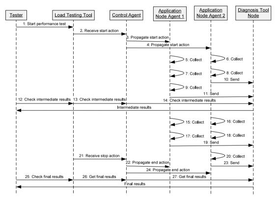
Figure 7. PHOEBE - Sequence diagram.
