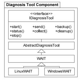
Figure 6. Diagnosis Tool Component - Class Diagram.
