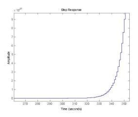
FIGURE 11 – The "Chernobyl phenomenon" (automated decision making system with real poles outside the unit circle) (unstable system).
