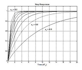
FIGURE 5 – Step responses of the discrete-time system given in Eq. 7 for different values of  $a_1$  and  $[b_1/(1 + a_1)] = 1$ .
