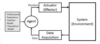
FIGURE 1 – Principle of DDDM (Data Driven Decision Making).
