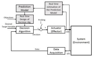
FIGURE 3 – Principle of adaptive automated MBDM (Data Driven Model Based Decision Making).
