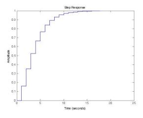
FIGURE 8 – Response of the automated model based desicion making for the case of real closed loop poles located inside the unit circle.
