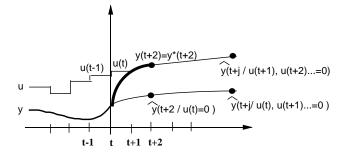
FIGURE 12 – Illustration of one step ahead predictive decision algorithm .
