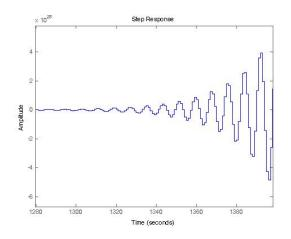
FIGURE 10 – Response of the automated model based decision making for the case of complex closed loop poles located outside the unit circle (unstable system).
