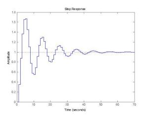
FIGURE 9 – Response of the automated model based desicion making for the case of complex closed loop poles located inside the unit circle.
