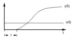
FIGURE 4 – Response of a system featuring a dead time  $(\tau)$  and an inertia.
