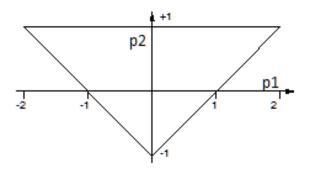
FIGURE 7 – Stability domain for a second order characteristic equation.
