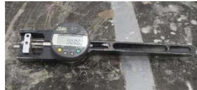
DEmountable MEChanical strain gauge
