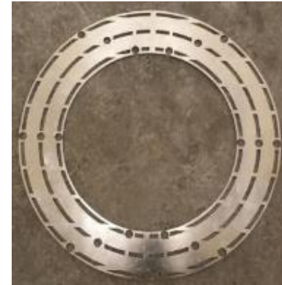
Template for positioning of the DEMEC
