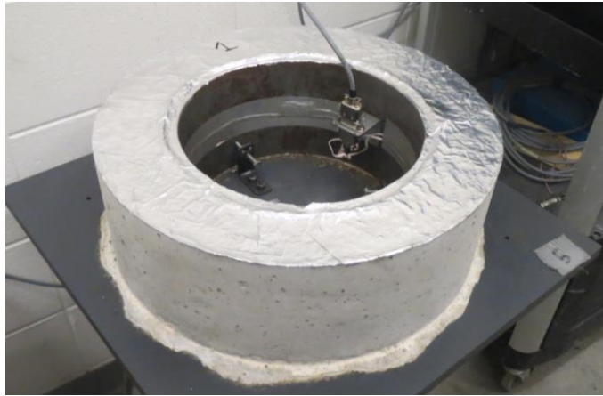
Restrained ring specimen
