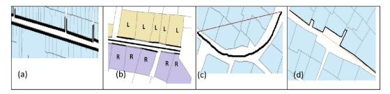
Fig. 5. (a) An edge with no cuts and the other with three cuts, (b) the parcels in two sides of a path to assess its symmetry, (c) path with bend and its substitute straight line, and (d) an unaligned edge and its substitute straight line.
