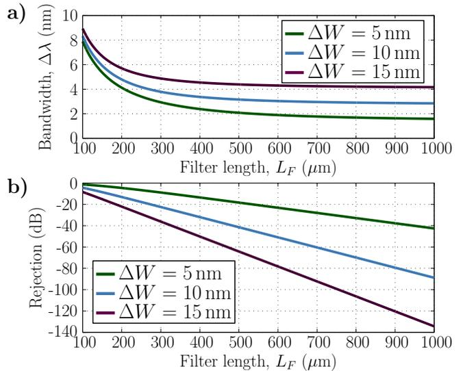
FIG. 4. Estimated (a) rejection bandwidth and (b) transmission level at center wavelength,  $\lambda_o$ , for double-periodicity Bragg filter as a function of the length,  $L_F$ , for various differential widths,  $\Delta W$ .
