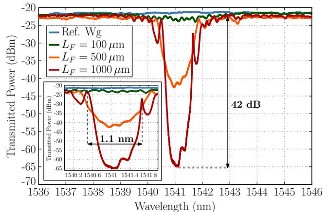
FIG. 6. Measured transmission spectrum of reference strip waveguide of  $1000 \mu\text{m}$  length and double-periodicity filters with differential width of  $\Delta W = 5 \text{ nm}$  and different filter lengths,  $L_F$ .
