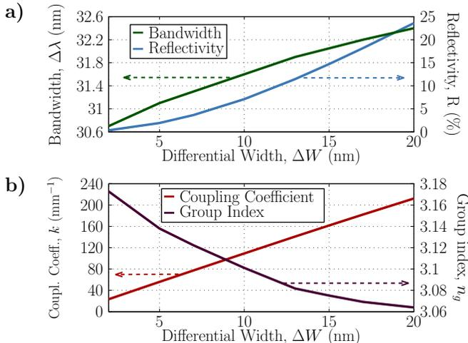
FIG. 3. Calculated (a) reflectivity and bandwidth, and (b) group index and coupling coefficient as a function of the differential width ( $\Delta W$ ) for a double-periodicity Bragg filter with  $W_C = 300$  nm,  $W = 150$  nm and length of  $L_F = 25$   $\mu\text{m}$ .
