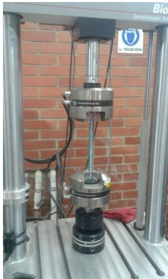
Figure 1. Tensile test on the MTS Bionix test machine for the composite pipe.
