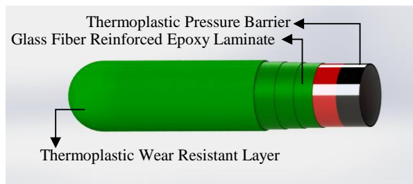
Figure 1. Fiberspar® pipe, construction model.
