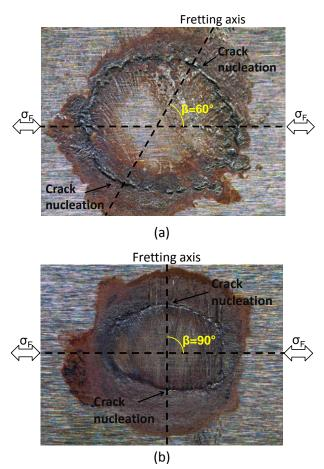
Figure 7: Fretting scars in multiaxial fretting fatigue after  $10^6$  cycles. (a)  $\beta$ =60°, Q\*=2700N; (b)  $\beta$ =90°, Q\*=3100N. (R=200mm, P=5000N,  $\sigma_{E,max}$ =400MPa,  $R_{\sigma}$ =0.8,  $10^6$  cycles).
