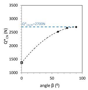
Figure 9: Crack nucleation conditions as functions of angle  $\beta$  (R=200mm, P=5000N,  $\sigma_{\text{F,max}}$ =400MPa,  $R_{\sigma}$ =0.8,  $10^6$  cycles). ( $\blacklozenge$ ) Non collinear FF crack nucleation conditions (NCFF test: centroid fatigue stress  $\rightarrow$  no eccentricity); ( $\blacksquare$ ) Collinear fretting fatigue crack nucleation condition (FF test: eccentricity).
