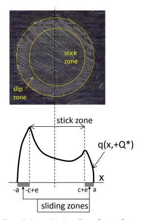
Figure 5: Eccentricity in collinear fretting fatigue
