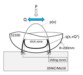
Figure 1: sketch of sphere on plane contact with partial slip; surface pressure profile p(x) (—) and surface shear profile q(x) (—).
