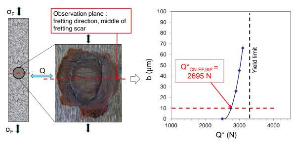
Figure 8: Illustration of the methodology used to identify the crack nucleation of non collinear fretting fatigue experiments (R=200mm, P=5000N,  $\sigma_{F,max}$ =400MPa,  $R_{\sigma}$ =0.8,  $10^6$  cycles,  $\beta$ =90°)
