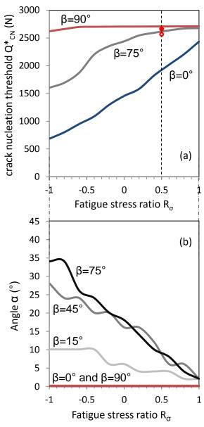
Figure 15: (a) evolution of crack nucleation threshold  $Q^*_{CN}$  as a function of the fatigue stress ratio  $R_\sigma$ . Comparison with experiments at  $10^6$  cycles for  $\beta$ =75°; •: crack nucleation (b=50 $\mu$ m); •: no crack nucleation. (b) Related evolution of the  $\alpha$ -angle with the x fretting axis direction where the first crack is nucleated (r/a=1,  $\theta$ =45° and  $\varphi$ =90°). (R=200mm, P=5000N,  $\sigma_{Fmax}$ =400MPa).
