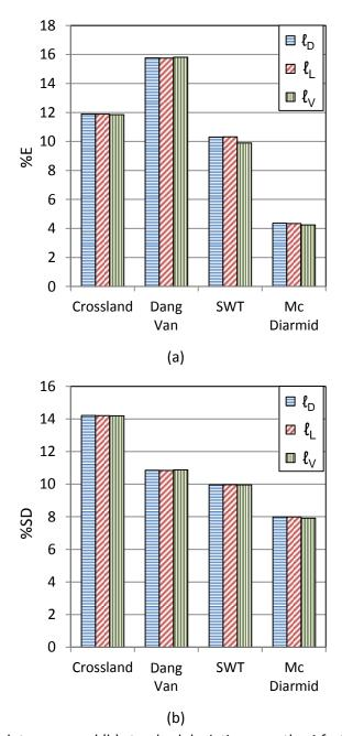
Figure 12: (a) mean absolute error and (b) standard deviation over the 4 fretting fatigue loadings at 4 different  $\beta$  angles considering 12 various criterion/length-scale combinations. (P=5000N,  $\sigma_{\text{F.max}}$ =400MPa,  $R_{\sigma}$ =0.8,  $10^6$  cycles).
