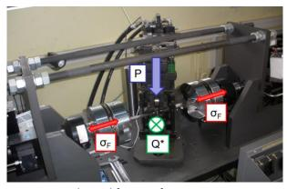
Figure 3: Multiaxial fretting fatigue set-up at LTDS.
