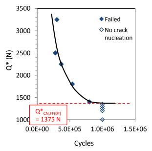
Figure 6: Identification of crack nucleation condition under collinear fretting fatigue loading  $\beta$ =0° (R=200mm, P=5000N,  $\sigma_{F,max}$ =400MPa,  $R_{\sigma}$ =0.8,  $10^6$  cycles).
