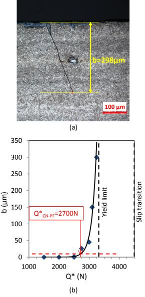
Figure 4: (a) Observation and measurement of crack length with optical microscope (R=200mm, P=5000N, Q\*=2700N,  $10^6$  cycles). (b) Identification of crack nucleation condition ( $b_{CN}$ = $10\mu$ m) under plain fretting loading (R=200mm, P=5000N,  $10^6$  cycles).
