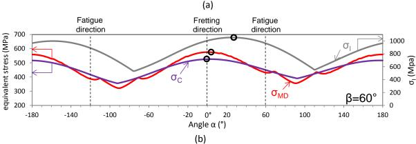
Figure 10: (a) XY mapping of  $\sigma_{\text{I}}$ , Crossland, Mc Diarmid as function of fretting fatigue loading and localization of maximum cracking risk. (b)  $\sigma_{\text{I}}$ , Crossland, Mc Diarmid evolution along the contact border for  $\beta$ =60°. (R=200mm, P=5000N, Q\*<sub>CN</sub>,  $\sigma_{\text{F,max}}$ =400MPa, R $_{\sigma}$ =0.8, 10<sup>6</sup> cycles).
