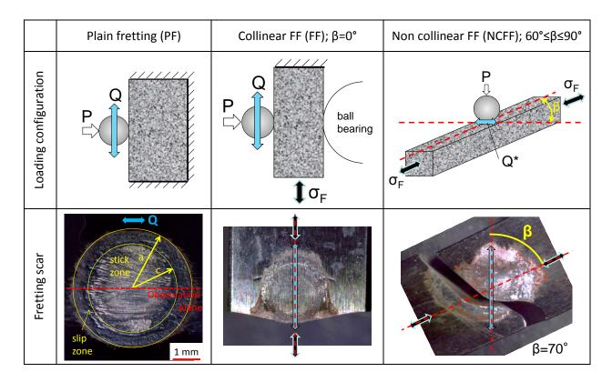
Figure 2: Loading configurations and related fretting scars for the three test configurations: plain fretting, conventional collinear fretting fatigue and on collinear fretting fatigue. (R=200mm, P=5000N, Q\*=2700N,  $\sigma_{F,max}$ =400MPa,  $R_{\sigma}$ =0.8,  $10^6$ cycles).  $\Longrightarrow$ : Fretting loading direction;  $\Longrightarrow$ : fatigue loading direction.
