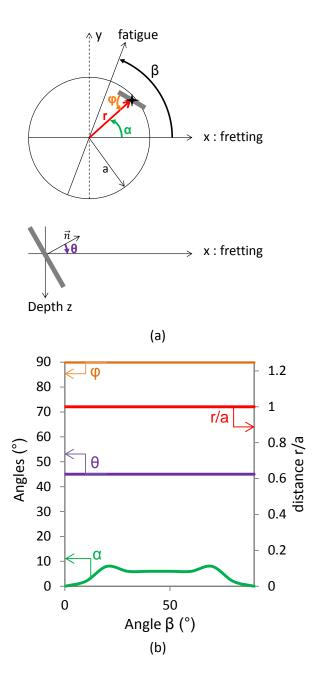
Figure 14: (a) Definition of parameters r,  $\alpha$ ,  $\theta$  and  $\phi$  for crack nucleation localization and critical plane orientation. (b)Evolution of the four parameters as functions of  $\beta$ . (R=200mm, P=5000N,  $\sigma_{F,max}$ =400MPa,  $R_{\sigma}$ =0.8).
