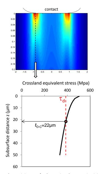
Figure 11: Identification of critical distance  $\ell_{\text{D-C}}$  from subsurface Crossland distribution (R=200mm, P=5000N, Q\*=2700N).
