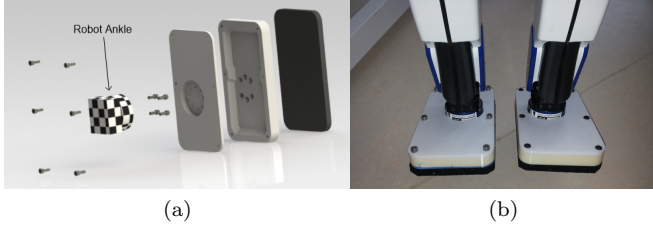
Figure 8: (a): new HRP-4's feet; (b): photo of HRP-4's feet with flexible soles
