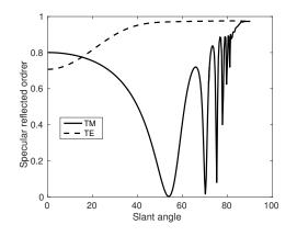
Figure 6: Specular reflected order versus slant angle for a dielectric grating enlightened under normal incidence in TE polarization and in TM polarization.  $w = 0.5, d = 1, h = 0.5, \lambda = 1.1, \epsilon_{21} = 1, \epsilon_{22} = (0.22 - i * 6.71)^2$ . The grating is suspended in air. The effective permittive is  $-21.9878 - i \times 1.4762$ . The reflectivity of the corresponding effective slab is 0.9731. We obtain the same value with a slant angle of  $89.99^{\circ}$
