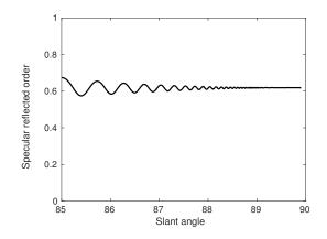
Figure 5: Specular reflected order versus slant angle for a dielectric grating enlightened under normal incidence in TM polarization.w = 0.5, d = 1, h = 0.5,  $\lambda = 1.1$ ,  $\epsilon_{21} = 1$ ,  $\epsilon_{22} = 25 - i0.0001$ . The grating is suspended in air. The effective permittive is 13. The reflectivity of the corresponding effective slab is 0.6191. We obtain the same value with a slant angle of 89.99°
