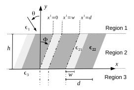
Figure 1: Geometry of the problem and illustration of the change of coordinates.  $\epsilon_1 = \nu_1^2, \epsilon_3 = \nu_3^2$
