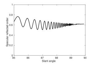
Figure 4: Specular reflected order versus slant angle for a dielectric grating enlightened under normal incidence in TE polarization. w = 0.5, d = 1, h = 0.5,  $\lambda = 1.1$ ,  $\epsilon_{21} = 1$ ,  $\epsilon_{22} = 25 - i0.0001$ . The grating is suspended in air. The effective permittive is 13. The reflectivity of the corresponding effective slab is 0.6191. We obtain the same value with a slant angle of  $89.99^{\circ}$
