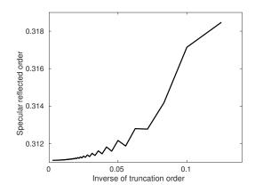
Figure 3: Convergence plot of the specular reflected order of a metallic grating in TM polarization
