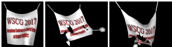
Figure 14: A cloth simulated in real-time (mass = 100g, stretching stiffness = 60  $N/m$ , shear stiffness = 43  $N/m$ , bending stiffness = 10  $N/m$ , damping = 0.1, fracture threshold = 0.5  $N$ ), using a global edge criterion.
