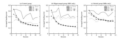
**Fig. 8.** Average heading error near the current platform for the three groups. Zero means the expert is pointing to the platform, one means a difference of  $\pi$ . (a) Results in the Control group (MBe and MFe activated) (b) Hippocampal group (MFe only) (c) Striatal group (MBe only).
