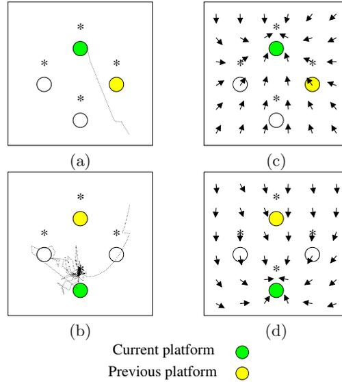
**Fig. 10.** (a) Trajectory at the fourth trial of the 7<sup>th</sup> session: as the simulated robot mainly went to this platform from the South, direction to the North were reinforced, even at the North of the platform.
