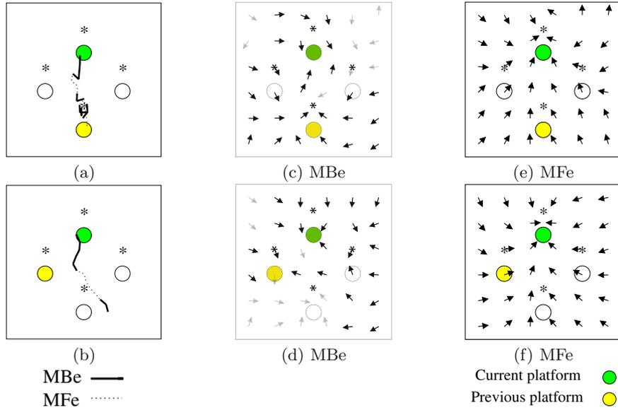
**Fig. 7.** Fourth trials: (a) Trajectory of the robot for the 3<sup>rd</sup> session (b) Trajectory of the robot for the 11<sup>th</sup> session. (c) Navigational map of the MBe for the 3<sup>rd</sup> session (d) Navigational map of the MBe for the 11<sup>th</sup> session (e) Navigational map of the MFe for the 3<sup>rd</sup> session (f) Navigational map of the MFe for the 11<sup>th</sup> session.
