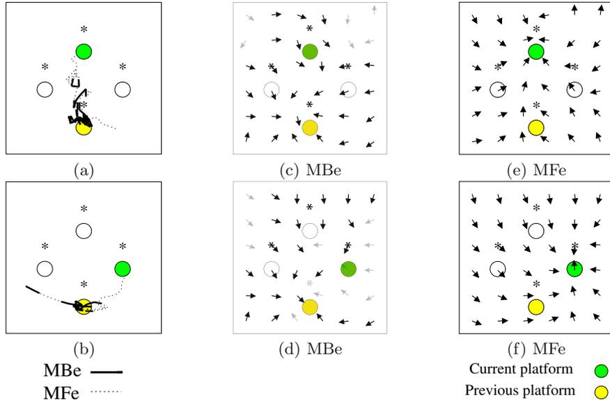
**Fig. 5.** First trials: (a) Trajectory of the robot for the 3<sup>rd</sup> session (b) Trajectory of the robot for the 9<sup>th</sup> session. (c) Navigational map of the MBe for the 3<sup>rd</sup> session (d) Navigational map of the MBe for the 9<sup>th</sup> session (e) Navigational map of the MFe for the 3<sup>rd</sup> session (f) Navigational map of the MFe for the 9<sup>th</sup> session.
