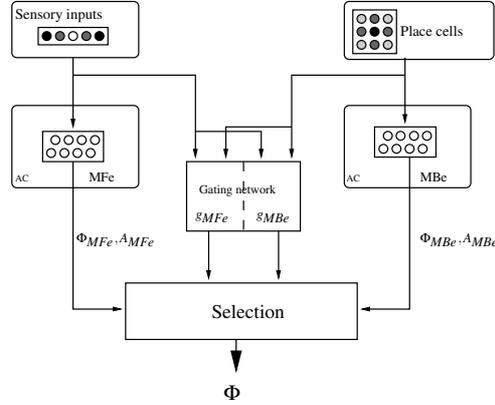
**Fig. 1.** The computational model of strategy selection [12]. The gating network receives the inputs of both experts, and their reward prediction error, in order to compute their reliability according to their performance (i.e., gating values  $g_k$ ). Gating values are then used with the Action value  $A_k$  in order to compute the probability of each expert to be selected. The direction  $\Phi$  proposed by the winning expert is then performed. See text for further explanations.
