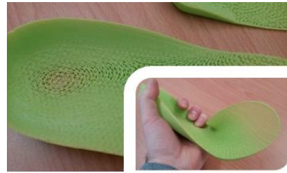
Figure 8. Different densities in the same insole
