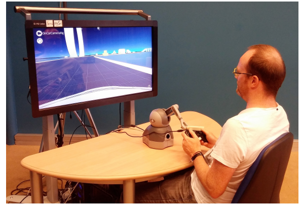
Figure 3: Proof-of-concept setup, based on a large screen and a gamepad attached to a 3DOF haptic device.
