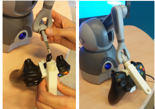
Figure 4: Assembly of the gamepad on the 3DOF haptic device with custom 3D printed holder and jack connector.
