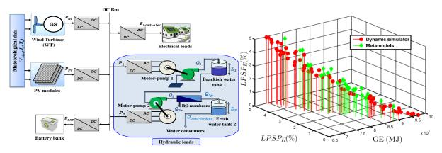
**Figure 1**. Three-objective optimization of the PV/Wind system with battery and two water tanks (*a*) system architecture (*b*) Pareto-optimal solutions issued from NSGA-II optimizations with the dynamic simulator and metamodels
