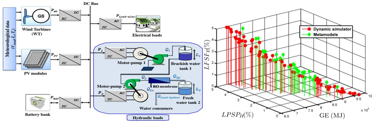
**Figure 1.** Three-objective optimization of the PV/Wind system with battery and two water tanks (a) system architecture (b) Pareto-optimal solutions issued from NSGA-II optimizations with the dynamic simulator and metamodels
