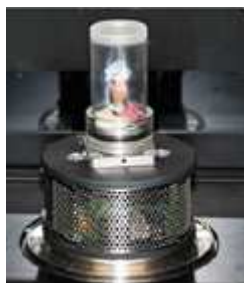
Figure 2. The cooling stage of the Skyscan 1172 system.
