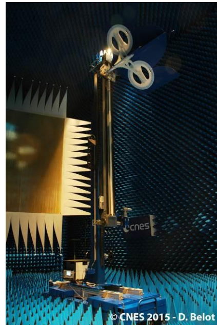
Figure 7. Photograph of the measurement probe in the measurement (expanded) configuration
