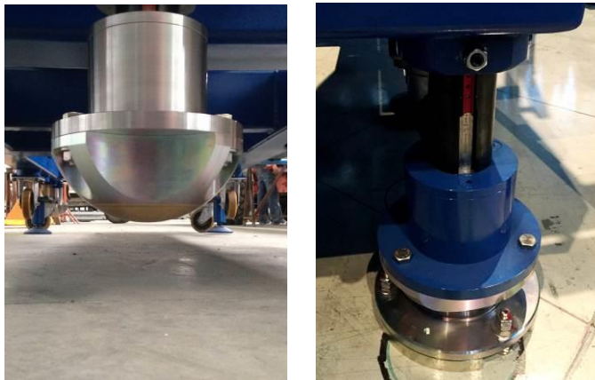
Figure 5. Integrated piston with anchor hemisphere and dedicated spherical container on the chamber floor
