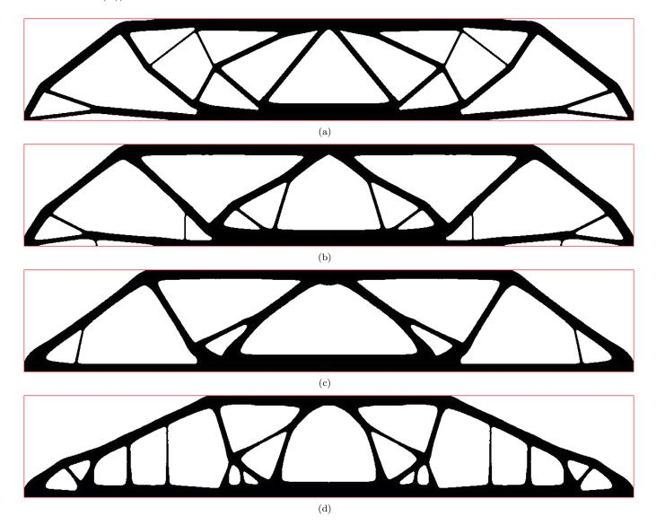
FIGURE 21. Optimized shapes for the two-dimensional MBB Beam example of Section 5.3.3: (a) optimized shape  $\Omega^*$  for Problem (5.3) (i.e. without additive manufacturing constraints), and optimized shapes for Problem (5.9) using parameters (b)  $\alpha_c = 0.50$ , (c)  $\alpha_c = 0.30$ , and (d)  $\alpha_c = 0.10$ .
