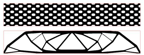
FIGURE 10. (Top) initial and (bottom) optimized shapes for Problem (5.3) in the twodimensional MBB Beam test-case of Section 5.2.2.
