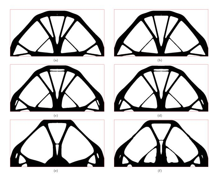
FIGURE 20. Optimized shapes in the two-dimensional bridge test case of Section 5.3.2 (left column) no acceleration procedure is used, and (a)  $\alpha_c = 0.7$ , (c)  $\alpha_c = 0.5$  and (e)  $\alpha_c = 0.3$ ; (right column) the acceleration procedure is used and (b)  $\alpha_c = 0.7$ , (d)  $\alpha_c = 0.5$  and (f)  $\alpha_c = 0.3$ .
