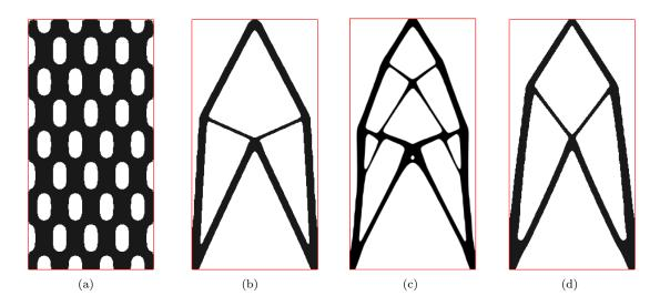
FIGURE 8. Penalization of the overhang features in the 2d cantilever of Section 5.2.1 using geometric constraints: (a) initial shape  $\Omega^0$ , (b) optimized shape  $\Omega^*$  for Problem (5.3), (c) optimized shape for Problem (5.4) using  $\varphi = \varphi_a$ ,  $\nu = 45^\circ$ , and  $\alpha_g = 0.01$ , (d) optimized shape using  $\varphi = \varphi_p$ ,  $\alpha_g = 0.02$  and the patterns defined by (5.5).
