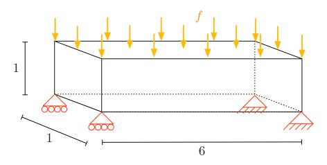
FIGURE 28. Setting of the three-dimensional bridge test-case.
