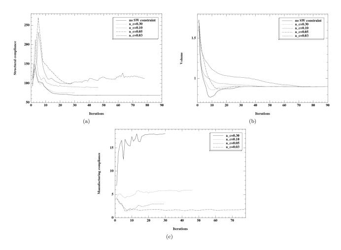
FIGURE 24. Convergence histories associated to the two-dimensional MBB Beam optimization example of Section 5.3.3, leading to the optimized shapes in Figure 23: (a) structural compliance  $J(\Omega)$ , (b) volume Vol( $\Omega$ ), and (c) upper-weight manufacturing compliance  $P_{uw}(\Omega)$ .
