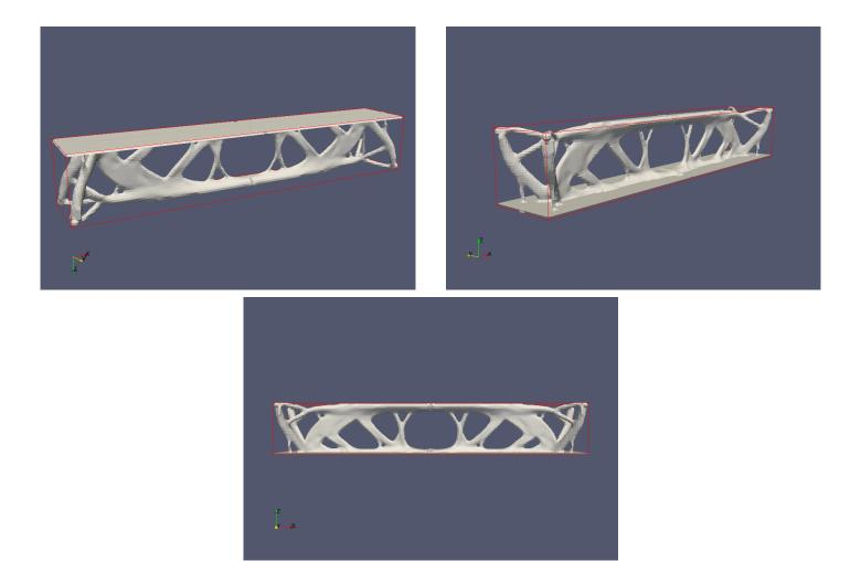
FIGURE 35. Optimized shape for the three-dimensional bridge example for the combined geometrically and mechanically constrained Problem (5.14) setting  $\alpha_c = 0.70$ ,  $\alpha_g = 0.10$ .
