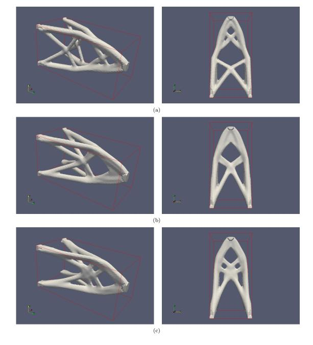
FIGURE 26. Optimized three-dimensional cantilever in the test-case of Section 5.4.1, solving Problem (5.11) (a) without additive manufacturing constraints, (b) using  $\alpha_c = 0.90$ , and (c) using  $\alpha_c = 0.70$ .
