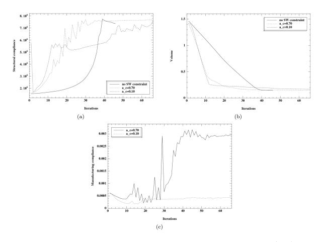
FIGURE 31. Convergence histories for the three-dimensional bridges of Figures 29 (right) and 30; (a) structural compliance  $J(\Omega)$ , (b) volume  $Vol(\Omega)$ , and (c) upper-weight manufacturing compliance  $P_{uw}(\Omega)$ .
