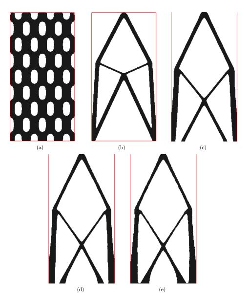
FIGURE 15. Optimized two-dimensional cantilever beams under the self-weight manufacturing compliance constraint  $P_{\rm sw}(\Omega)$ , in the setting of Section 5.3.1: (a) initial shape  $\Omega^0$ , (b) optimized shape  $\Omega^*$  for Problem (5.3) (i.e. without additive manufacturing constraints), and optimized shapes for Problem (5.9) using the parameter (c)  $\alpha_c = 0.80$ ; (d)  $\alpha_c = 0.60$ ; (e)  $\alpha_c = 0.50$ .
