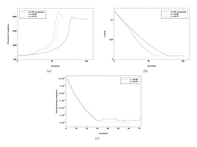
FIGURE 27. Convergence histories for the optimized three-dimensional cantilever beams of Figure 26: (a) structural compliance  $J(\Omega)$ , (b) volume  $Vol(\Omega)$ , and (c) upper-weight manufacturing compliance  $P_{uw}(\Omega)$ .
