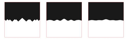
FIGURE 13. Optimized shapes for the purely geometric Problem (5.7) under perimeter penalization, using the values (from left to right)  $\ell = 0.01$ , 1 and 10.
