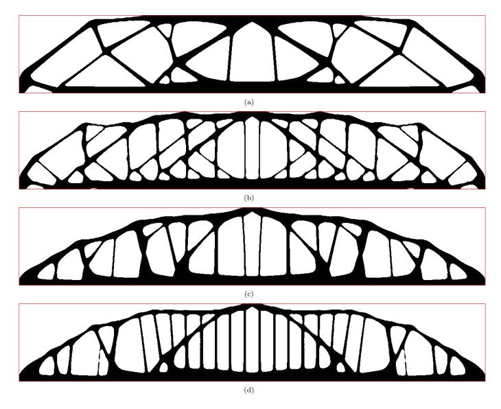
FIGURE 23. Optimized shapes for the two-dimensional MBB Beam example of Section 5.3.3, solving Problem (5.9) with the upper-weight manufacturing compliance  $P_{uw}(\Omega)$  and parameters (a)  $\alpha_c = 0.30$ , (b)  $\alpha_c = 0.10$ , (c)  $\alpha_c = 0.05$ , and (d)  $\alpha_c = 0.03$ .
