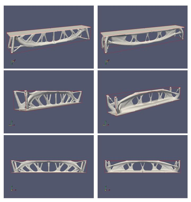
FIGURE 36. Optimized three-dimensional bridges for the combined geometrically and mechanically constrained Problem (5.14) setting (left)  $\alpha_c = 0.10$ ,  $\alpha_g = 0.10$ , and (right)  $\alpha_c = 0.10$ ,  $\alpha_g = 0.90$ .
