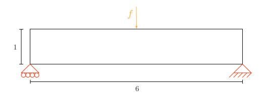
FIGURE 9. Setting of the two-dimensional MBB beam example.
