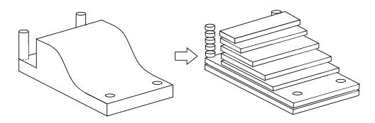
FIGURE 1. Rough sketch of the slicing procedure, initiating any additive manufacturing process.
