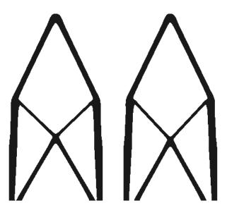
FIGURE 17. Optimized shapes for Problem (5.9) in the two-dimensional cantilever example of Section 5.3.1, when  $P_{sw}(\Omega)$  and  $\mathcal{D}_{\Omega}$  are approximated by (left)  $P_{200}^0$  and  $\mathcal{D}_{200}^0$ ; (right)  $P_{25}^1$ and  $\mathcal{D}_{25}^1$ .
