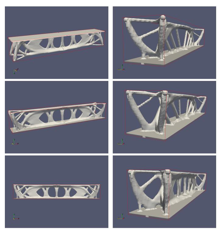
FIGURE 30. (Left) Different views of the optimized shape for the three-dimensional bridge example of Section 5.4.2, solving Problem (5.12) with  $\alpha_c = 0.1$ ; (right) another view on the three-dimensional bridges for Problem (5.12) with (top) no manufacturing constraint, (middle)  $\alpha_c = 0.7$  and (bottom)  $\alpha_c = 0.1$ .
