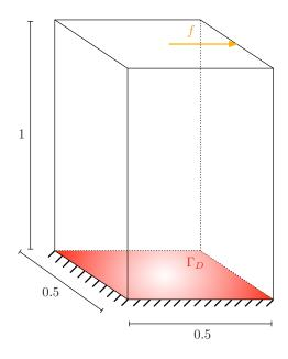
FIGURE 25. Setting of the three-dimensional cantilever test case.
