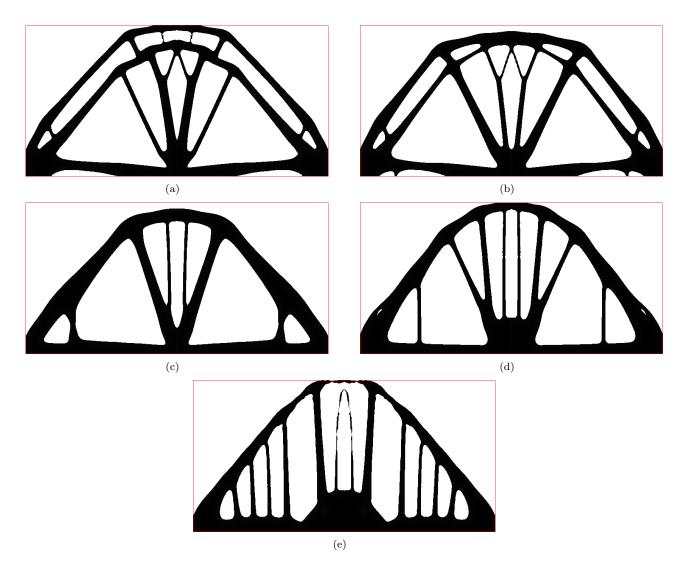
FIGURE 22. Optimized two-dimensional bridges using the upper-weight manufacturing compliance  $P_{uw}(\Omega)$ , and the parameters  $\alpha_v = 0.3$  and (a)  $\alpha_c = 0.7$ , (b)  $\alpha_c = 0.5$ , (c)  $\alpha_c = 0.3$ , (d)  $\alpha_c = 0.2$ , and (e)  $\alpha_c = 0.1$ .
