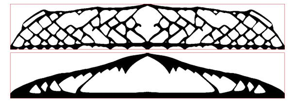
FIGURE 11. Optimized shapes resulting from Problem (5.4) in the two-dimensional MBB Beam example, using (top)  $\varphi \equiv \varphi_a$  and the threshold angle  $\nu = 45^\circ$ , and (bottom)  $\varphi \equiv \varphi_p$ and the pattern functions  $\psi_i$  defined in (5.5).
