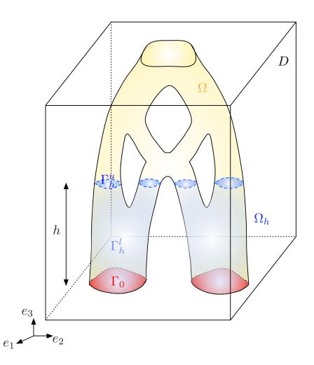
FIGURE 5. Physical setting of the shape  $\Omega$  during the additive manufacturing process.
