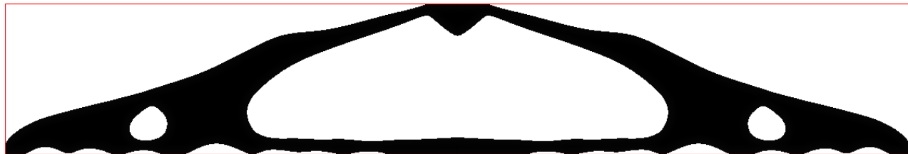
FIGURE 14. Optimized two-dimensional MBB Beam for Problem (5.8), under both a geometric and perimeter constraint.
