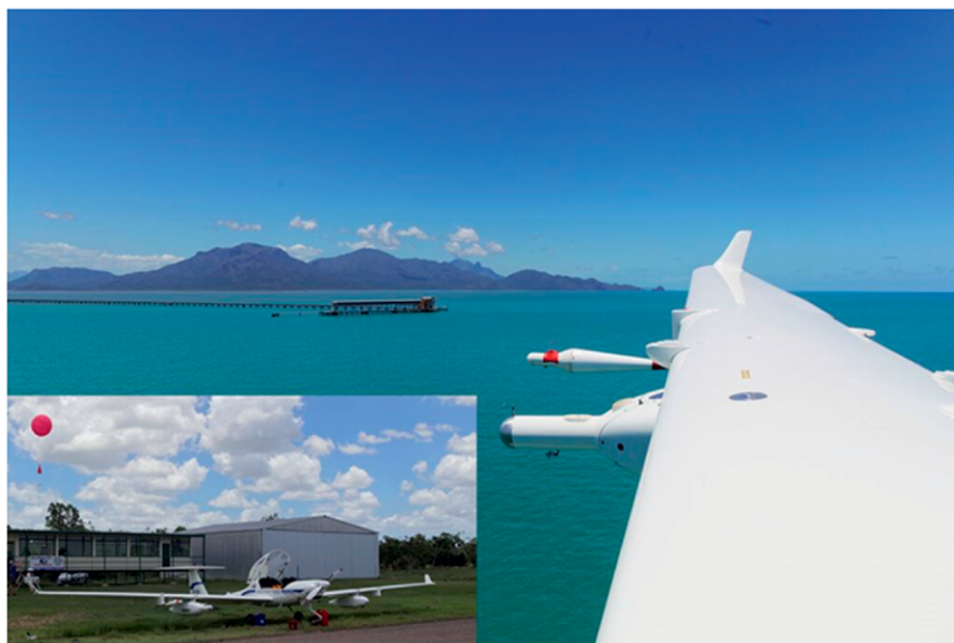
FIG. 7. The ECO-Dimona, flying past the Lucinda jetty during TAPS. Two air turbulence probes are seen mounted underneath the aircraft wing. (inset) The ECO-Dimona at Ingham Airfield. The instrument pods under the wings are clearly visible.
