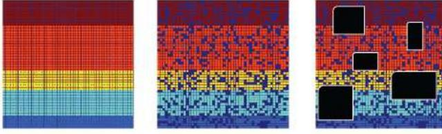
**Fig. 2** Illustration of different types of corruption for the matrix  $A$ : a)  $A$  without noise b)  $A$  with element-wise outliers/noise and c)  $A$  with both element-wise outliers/noise and missing data (Illustration from the slides of Ma et al. [208]).
