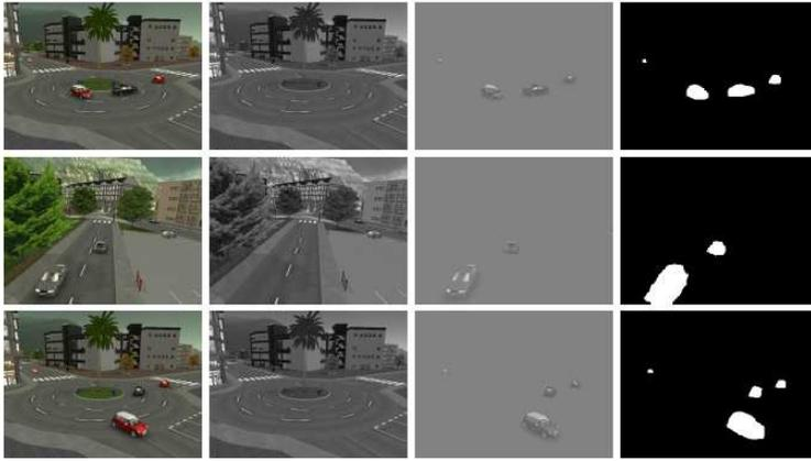
**Fig. 1** RPCA via decomposition into low-rank plus sparse matrices in foreground/background separation: Original image (309), low-rank matrix  $L$  (background), sparse matrix  $S$  (foreground), foreground mask (Sequences from BMC 2012 dataset [315]).
