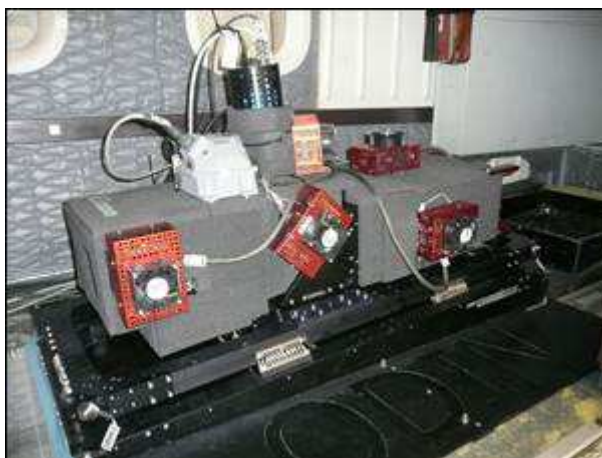
Figure 1. The HySpex ODIN-1024 spectral imager installed into the aircraft.
