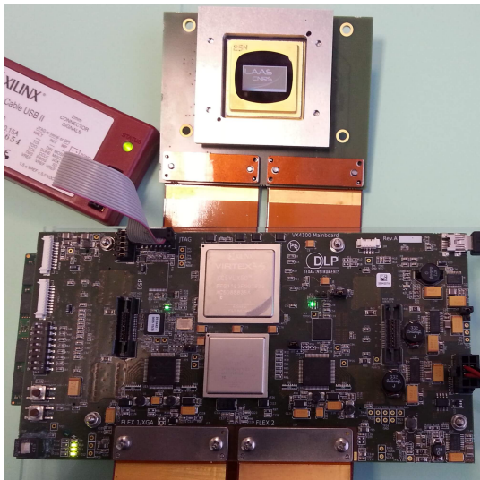
Fig. 6: FPGA board for tight loop control of both CMOS detector and micro-mirror array.
